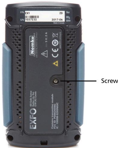
4. Remove the battery compartment door.
