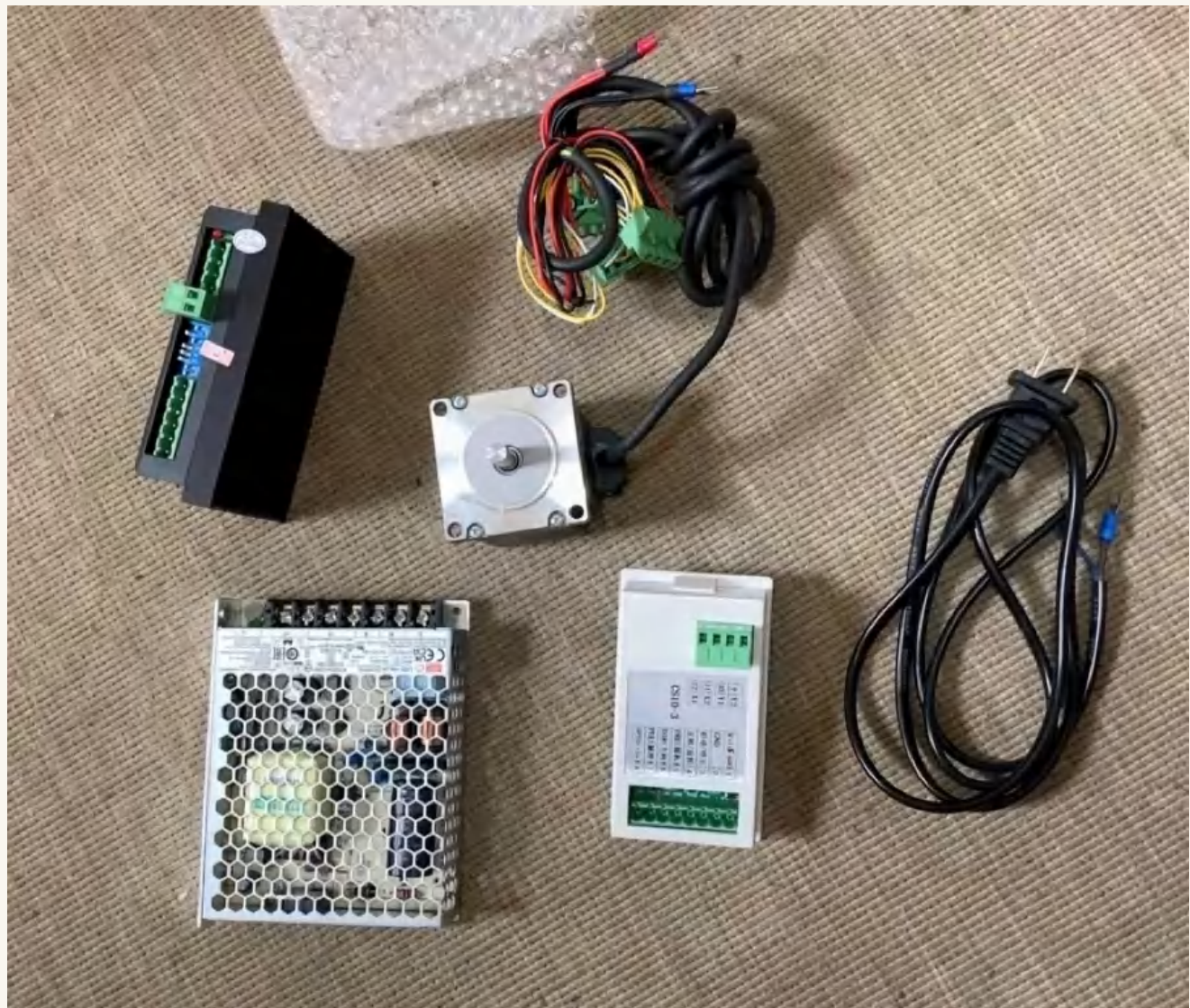
Electronic Components: Stepper Motor Pulse/ Generator Controller/ Power Transformer/ Stepper Motor Driver
