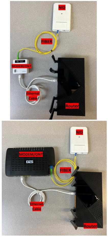
This is a NID usually mounted on the wall. The fiber is ran from outside to this box, from there it is connected to your modem/ONT: (you should **NEVER** unplug this from either the NID or modem)
