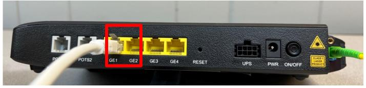
The other end of the Ethernet cable should plug in the WAN/Ethernet port only of the router.
