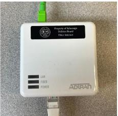
The ethernet cable should only be plugged into GE1 of the modem/ONT.
