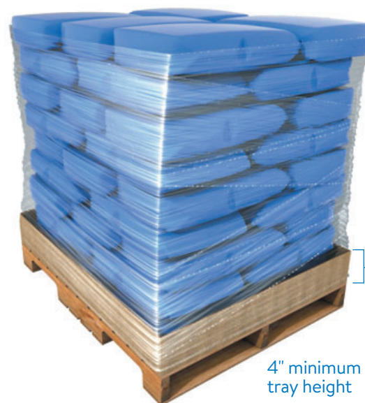
CORRECT (Interlocking with 4" bottom tray)
