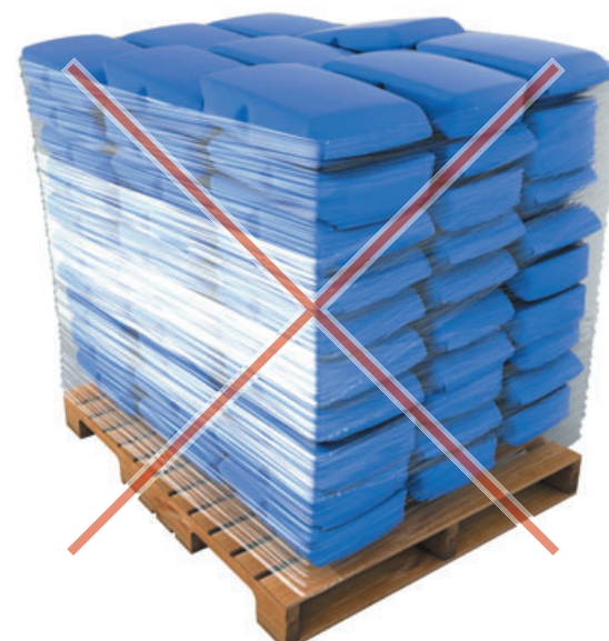
INCORRECT (Not interlocked, no bottom tray)
