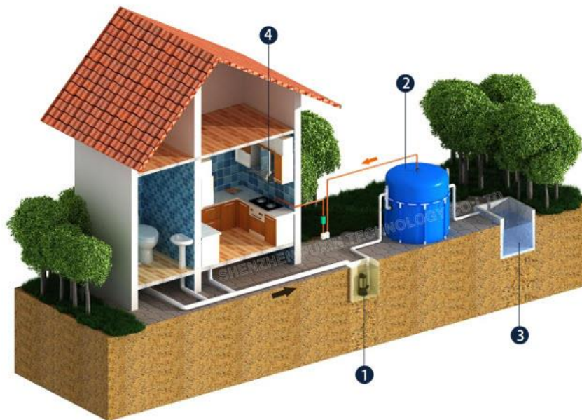
1.feeding pump, 2.digester, 3.slurry pool, 4.biogas stove
