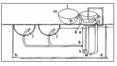
tank (ht) will empty itself through hole (t), float (z) will fall, valve (w) will close and pipes (jk) will discharge nothing and the water will remain in the bowls. Anyone looking at the wild animals will get the illusion that they have refrained from drinking when the lion refrained. And that is what we wished to explain.
