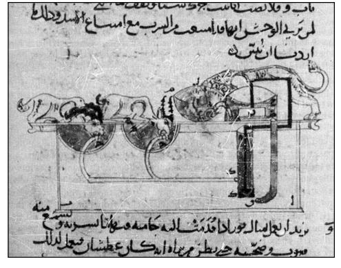
it overflows from edge (h) into plinth (ab). We make pipe (yk): its end (k) discharges into tank (ht) and its end (y) is soldered to the mouth of the lion. Tank (ht) is thus enclosed in the hollow of the lion so that it is hidden from view. From end (k) of pipe (ke) we lead out two pipes (k) and we place their ends marked (j) in the bottoms of the bowls and solder them to the mouths of the wild animals. It should be clear from our
