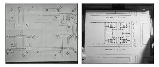
(Abstraction at work: a diagram showing the locations of the alarm system's clock stations in the office building. These need to be routinely punched by guards patrolling the premises; otherwise, the gear mechanism would wind up, turn a wheel with its teeth and pulse an emergency code to the police station—where officers would use index cards to identify the source of the signal)
