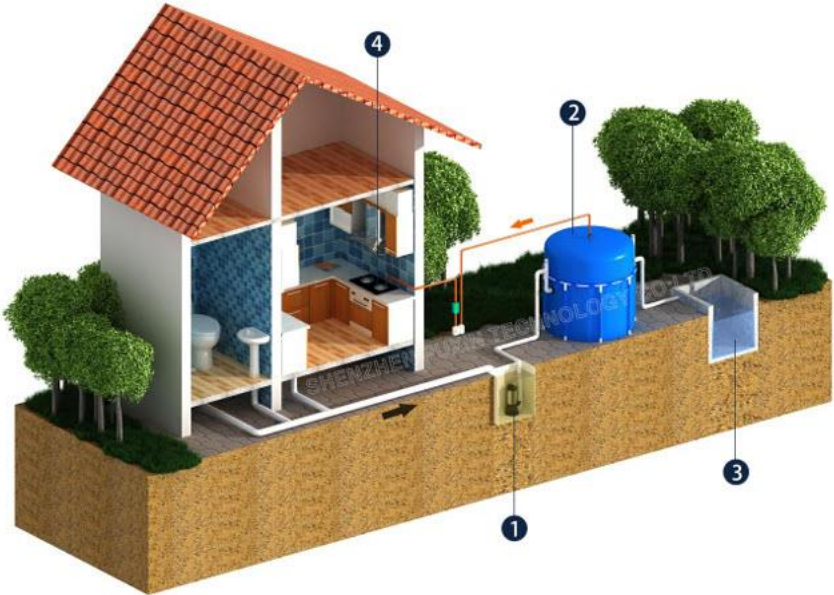
1.feeding pump, 2.digester, 3.slurry pool, 4.biogas stove
