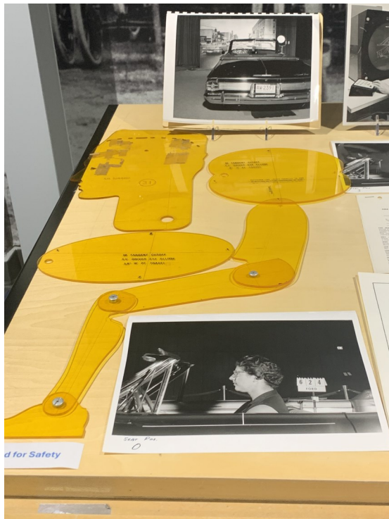
These silhouettes were used to configure seating positions and sizes for full size scale drawings
