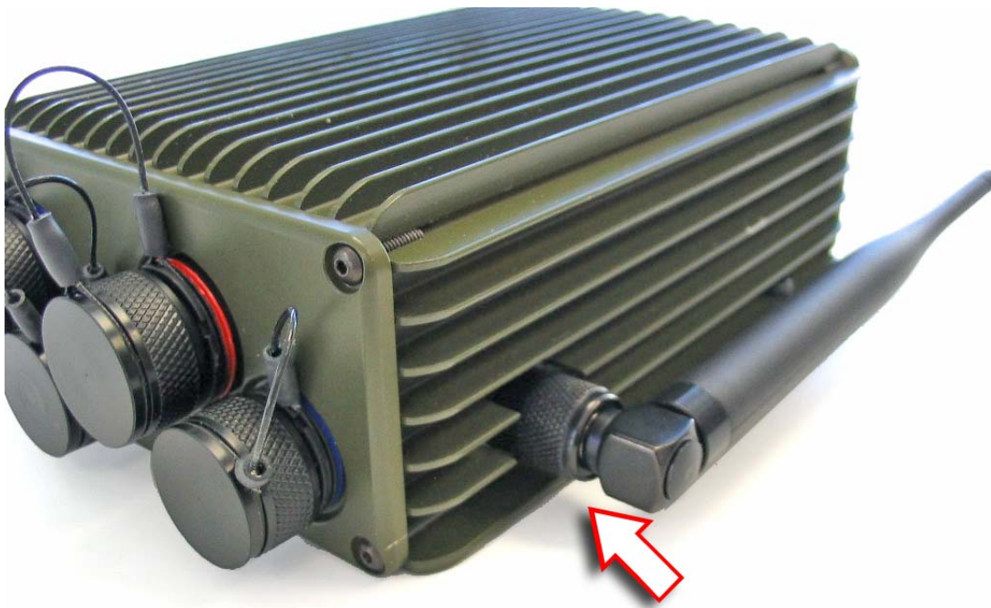
Figure 2-13 Connecting the external 802.11 antenna
