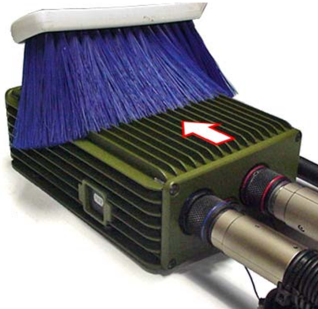
Figure 5-1 Brushing Thermite case fins
