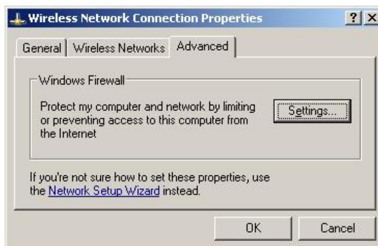
Figure 4-14 Firewall settings access
