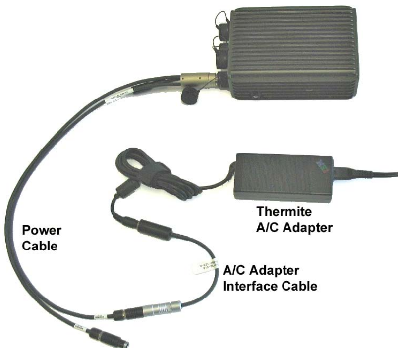
Figure 2-12 Thermite AC adapter connection
