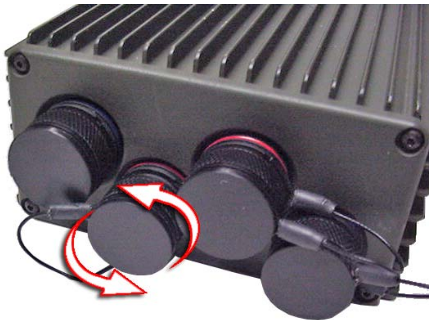
Figure 2-4 Unscrewing a waterproof cap
